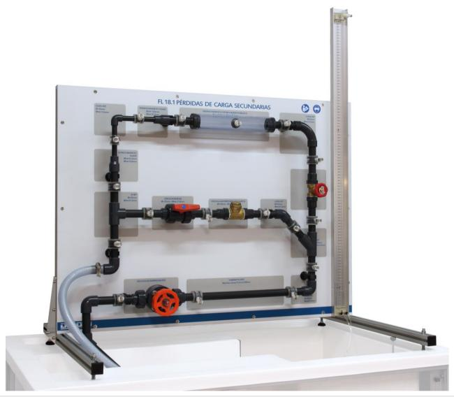
This installation for the study of the energy losses has elements such as; elbows of different diameters at 90° and 45°, tees, widening, narrowing, different types of valves (ball, gate, diaphragm, non-return,...) with upstream and downstream pressure tappings arranged for determination of the head loss between them, produced with different flow rates. It also has straight sections of pipe, which allows the study of the primary loss generated in it.
